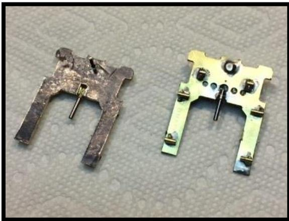
The pan is now ready. The wiper holders and torsion bar retainers will be installed during final assembly.
