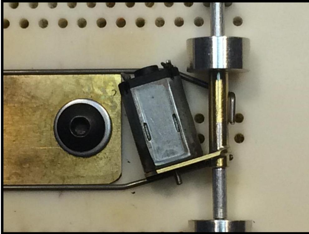
difficult. Start with the bend by the endbell of the motor. The rail must snake between the motor and the jig wheel. Remember the actual wheel will be larger than the jig wheel so to ensure clearance between the rail and the wheel, stay at least 0.030"
