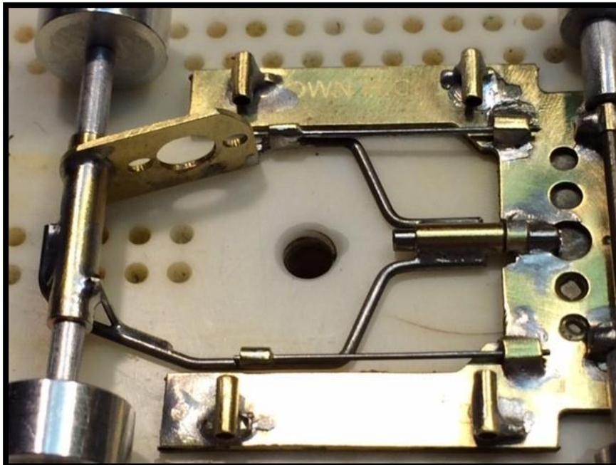
against the jig and the rails end up alongside the hinge tube. Ensure the hinge tube is up against the brass pin boss and solder the rails to the tube.
