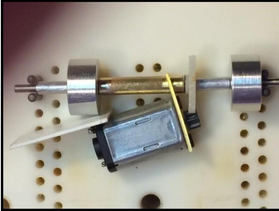
allow adequate clearance between the gear and the track rails. To ensure the motor won't rub against the rear wheels, use a 0.030" piece of plastic to space the motor away from the jig wheel. Align the motor bracket so the edge of the pinion lines up with the edge of the spur gear. The axle hole in the motor bracket will have to be opened up to
