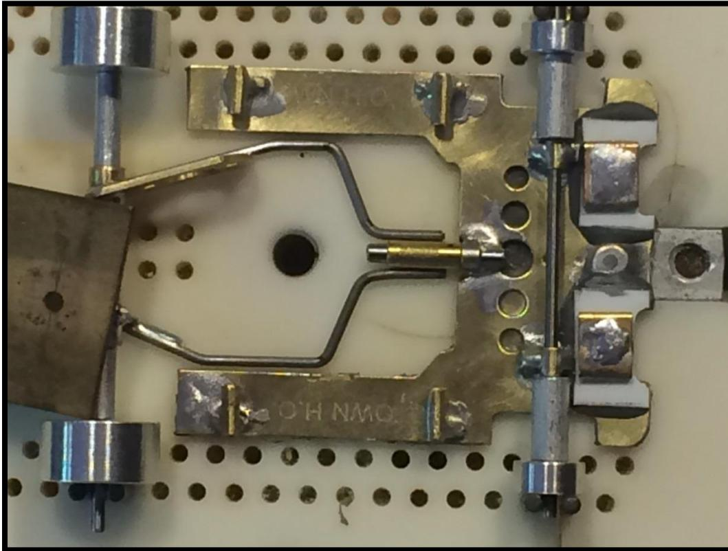
to bend the rails so they are properly aligned with the center hinge tube. The hardest part of this task is keeping the rails flat against the jig. Go slow, bend a little, trial fit and
