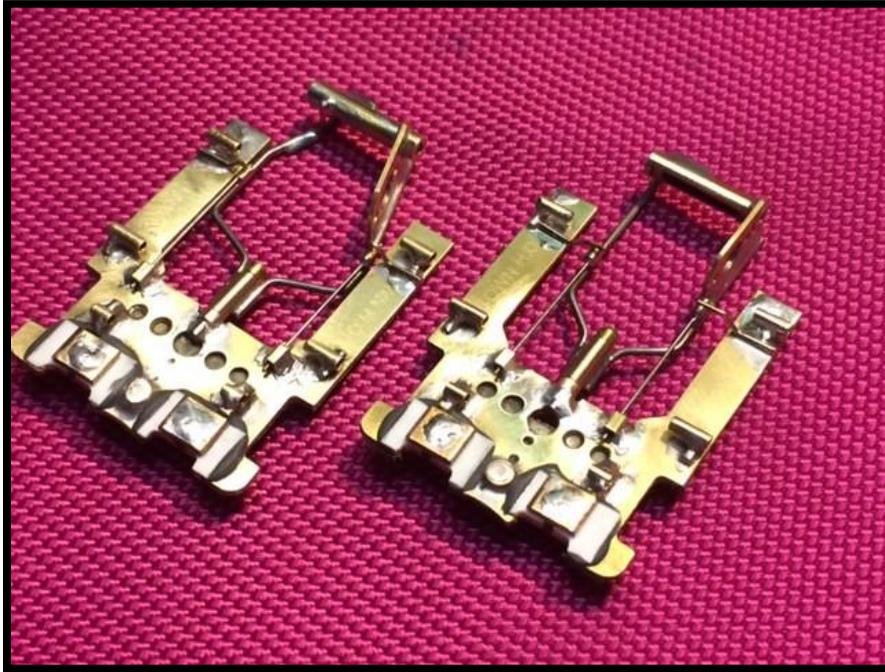
Now we can finish up the chassis by installing the small brass tube over the hinge pin to tie the front and rear of the chassis together. The brave amongst us might want to solder this tube in place but I worry about soldering wicking inside the pivot tube and soldering the hinge solid. I use a small drop of Loctite 620 to hold the cap in place. There's little load on this cap and the Loctite has worked fine thus far.
