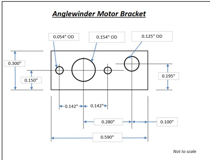
Let's start with the motor bracket. It is constructed using a 0.025" x 0.5" brass strip (K&S # 8236). Cut a piece approximately 1" long. Then layout the holes per the dimensions in the photo. Once the dimensions are lightly scribed onto the brass, use a center punch to locate the hole centers and, using a drill press, open the holes to their correct diameters. While accuracy is great, a small round jeweler's file will help correct any errors.
