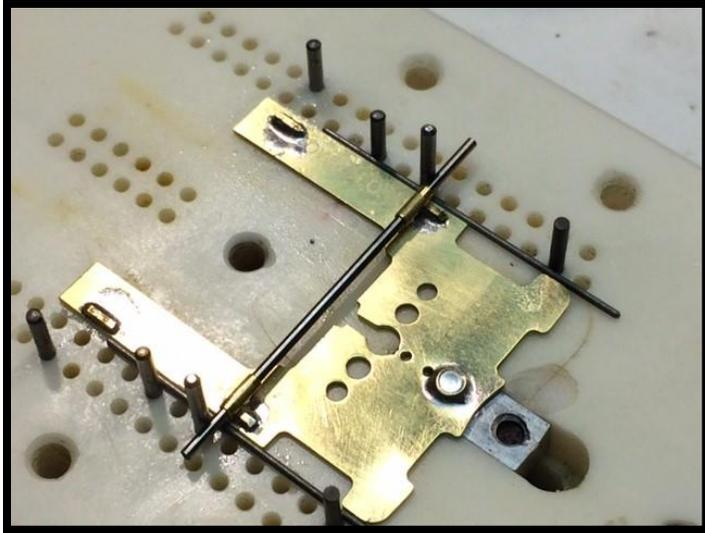
Next step is to solder short pieces of 1/32" square brass bar to the pan to space up the pin tubes properly. Then, using the chassis jig to keep things square, solder the pin tubes on top of the spacers using a piece of 3/64" piano wire to align the pin tubes.
