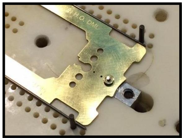
area being heated up. That's why starting here is important because other parts won't unsolder when heating up the pan for the guide pin installation. Center the pan on the jig using spare pieces of piano wire (if the pan has been narrowed). The jig should hold the guide pin square to the chassis while soldering.
