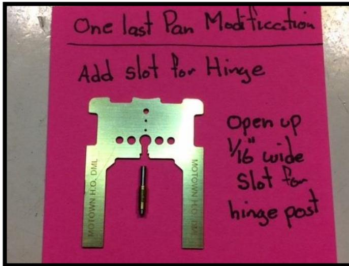
The last modification to the pan is to add a slot for the center-hinge pin; a Dremel tool and a #409 cut-off wheel will do the trick. These cut-off wheels shatter easily so wear eye protection but they do make a nice clean, narrow cut. Mark the center of the pan as shown in photo, cut a slot and then open the width to accommodate the hinge pin and brass tubing boss.
