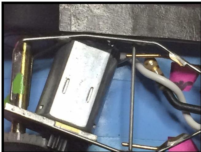
overall width that will pass through the tech block (1.312"). The front tires will need to be ground to 0.300", that should result in a 0.030" ground clearance. If the chassis is sitting much lower than 0.030", tweaking the wipers will be difficult; much higher than 0.030" and the center of gravity will be higher than desirable.
