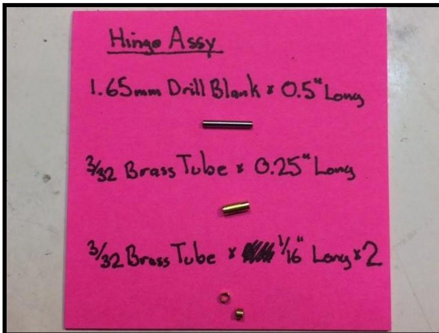
To fabricate the hinge assembly cut a piece of the 1.65mm drill blank a 1/2" long chamfering the ends slightly to remove the burrs. Next cut three pieces of 3/32" brass tube, one a 1/4" long and two pieces each approximately 1/16" long; remove the burrs from the inside and outside edges of the tubes. The rod and one of the short pieces of tubing will be soldered to the pan, the long piece of brass tube will be soldered to the motor frame with the second
