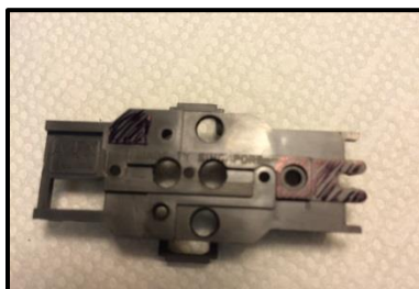
Areas marked where plastic needs to be removed
