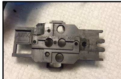
Modified chassis with plastic removed
