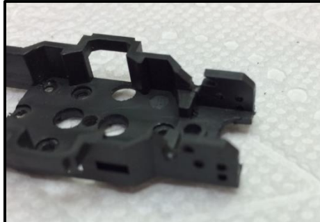
Adding grooves for floating pan cross-member, removing pickup shoe tabs and opening front of chassis for guide pin
