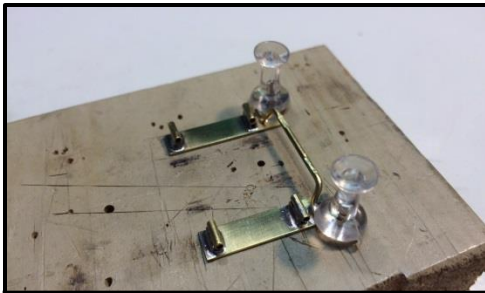
Soldering the pin tubes top the floating pan assembly clamping the cross member in place so it doesn't move if it gets unsoldered when adding the pin tubes
