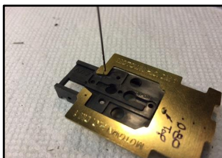
Tap the front hole while using the rear holes as a drill guide to properly locate the rear mounting screws
