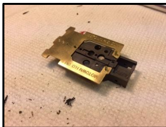
Ready for final measurements – tweak plastic removal as needed to ensure pan sits parallel to the top of the chassis
