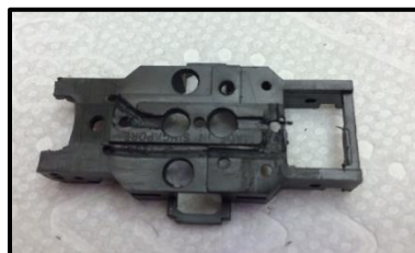
Modified chassis showing grooves for wire routing
